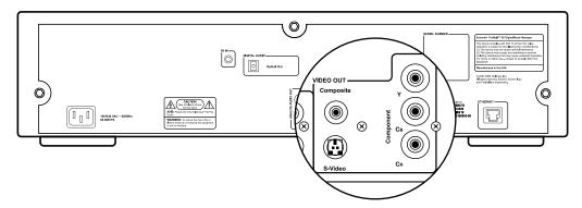
All video outputs are active at the same time, so you can use as many as you like without causing signal degradation.
